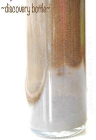
Eventually, as things settle, the heavy rocks/gravel will sink to the bottom, and then the sand will settle in a layer. A thin layer of grey clay will appear at last, and the organic material will remain floating or will settle on the top. The soil discovery bottle is a fun activity to do and to watch over the course of a week!
